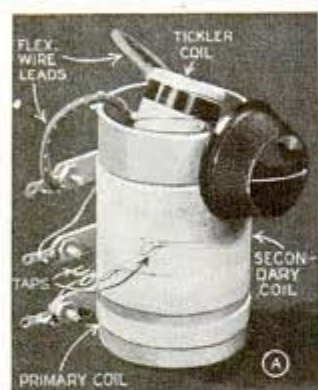
(A) Front view of completed 3-circuit tuner; (B) Rear view of terminal panel; (C) Schematic circuit diagram as used in 3-circuit receiver
